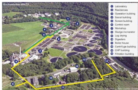
Figure 8-10: Heat grid at Buchenhofen
