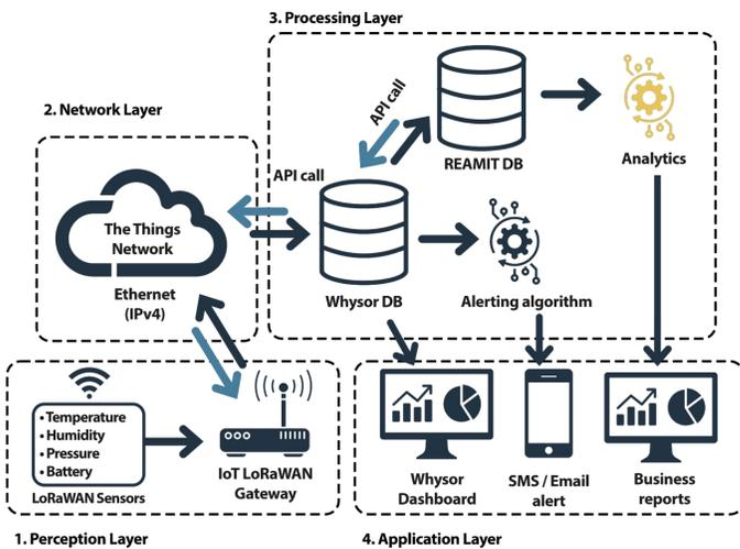
Figure 1. Example of REAMIT IoT architecture
