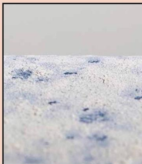
Surface of a conventional diatomaceous earth product, offering significantly flatter and smoother structures. This means shorter residence times for the mites on the surface and therefore an inferior effect.
