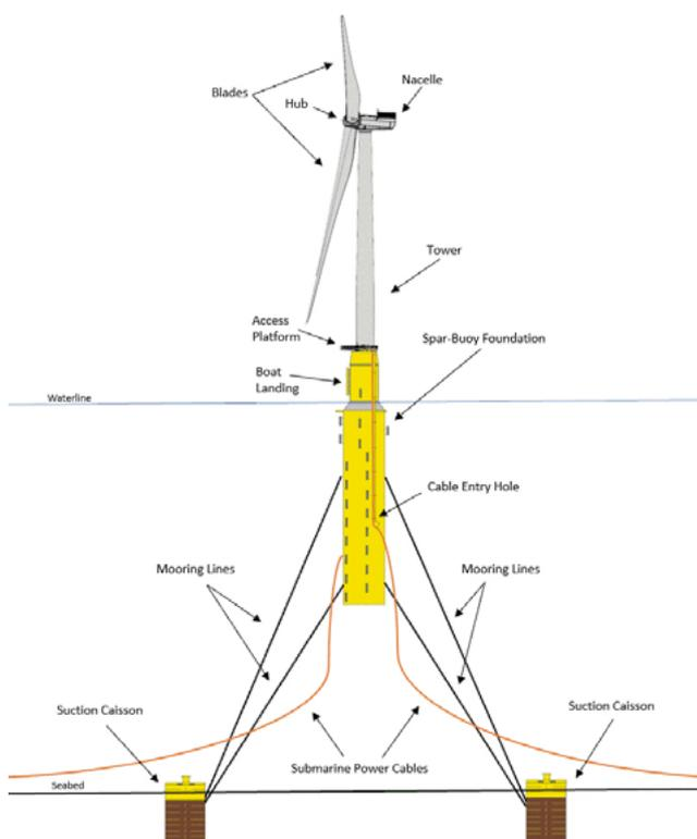
**Figure 8: Spar-buoy FOW turbine installed [15]**
