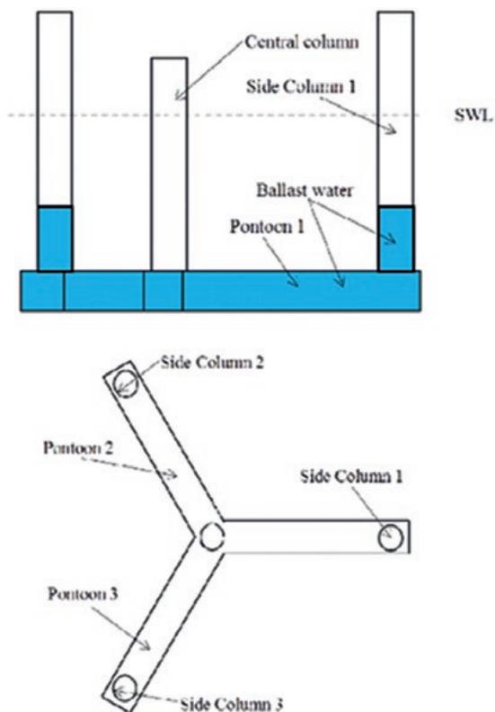
Similar to a barge-type platform, the semi-submersible platform can be constructed onshore or in a dry dock. Depending on the platform and wind turbine size and the capabilities of the yard, the complete turbine may be installed onto the platform at the quayside. The fully assembled system can then be towed out to the site using conventional tugs, avoiding the costly offshore installation.
