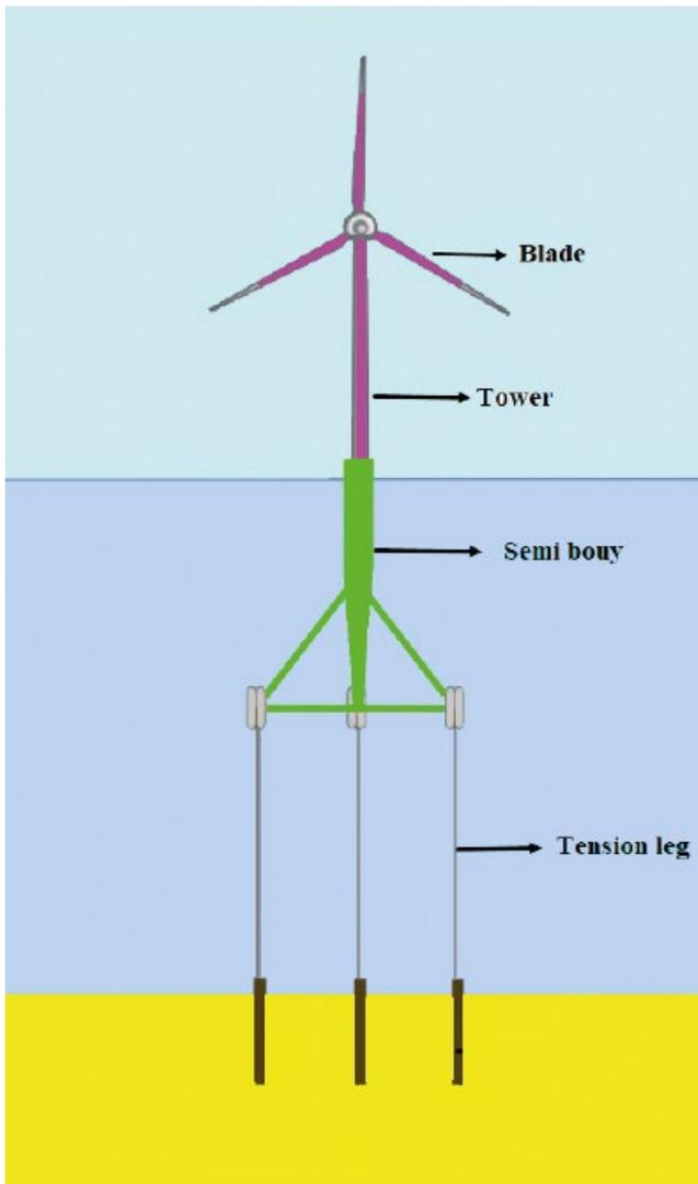
**Figure 10: Drawing of an installed tension-leg platform**
