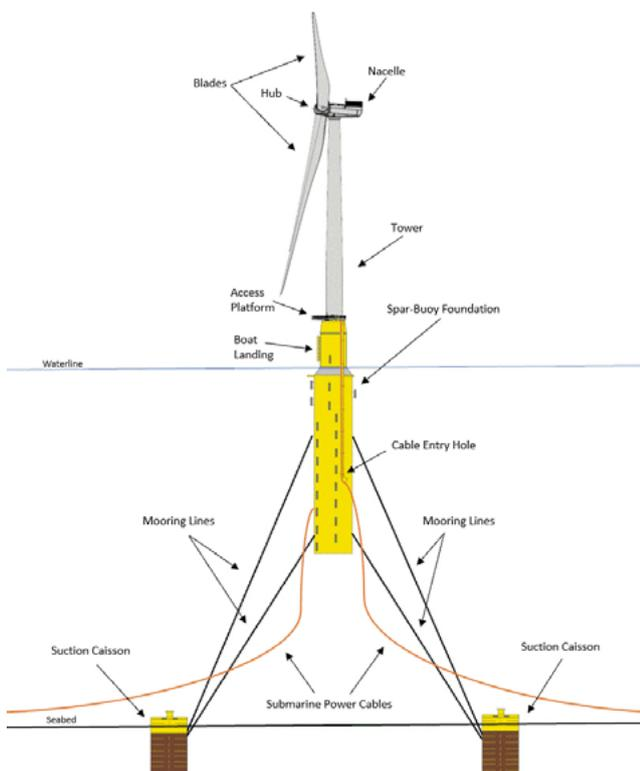
**Figure 8: Spar-buoy FOW turbine installed [15]**
