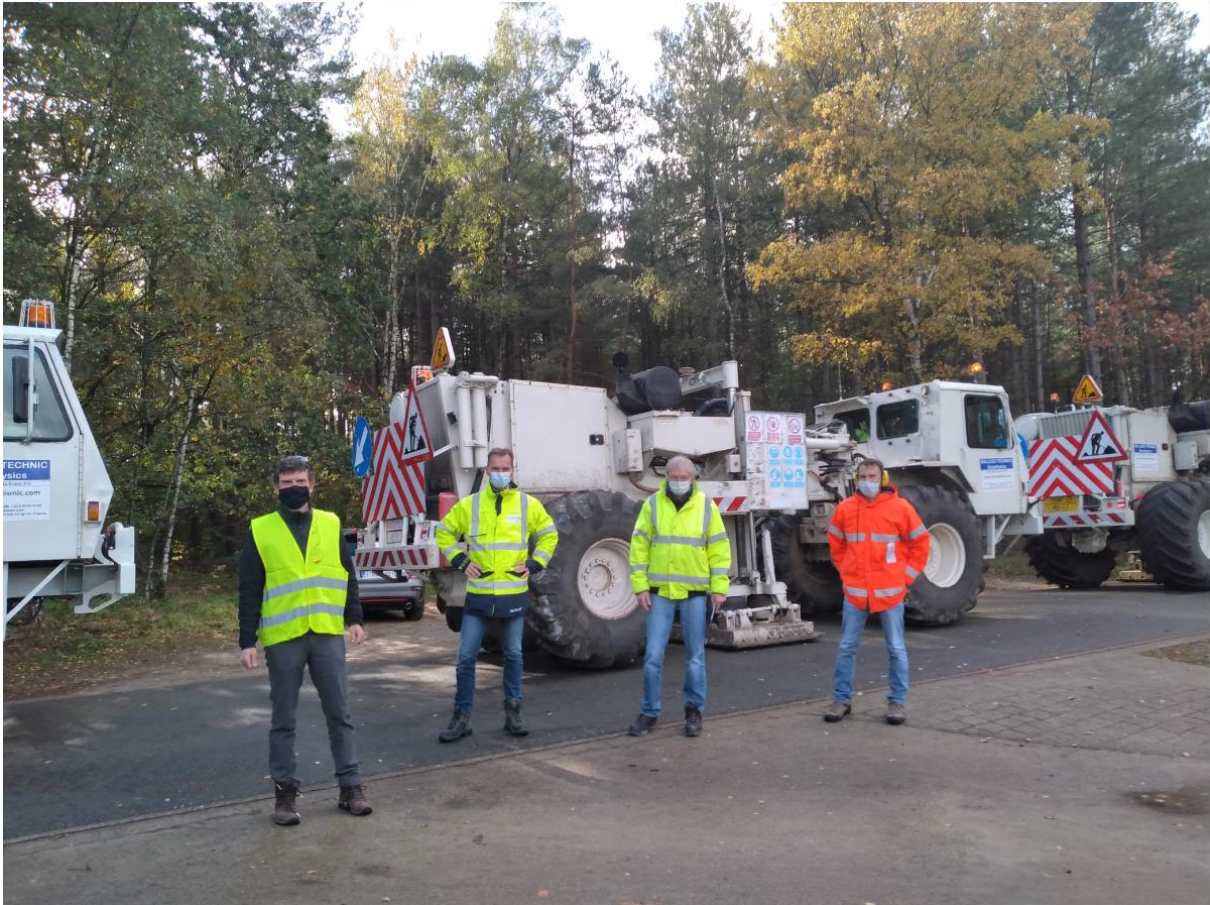
Figure 4: Vibration trucks in the field in Flanders – masks are related to COVID-19 measures in place at the time
