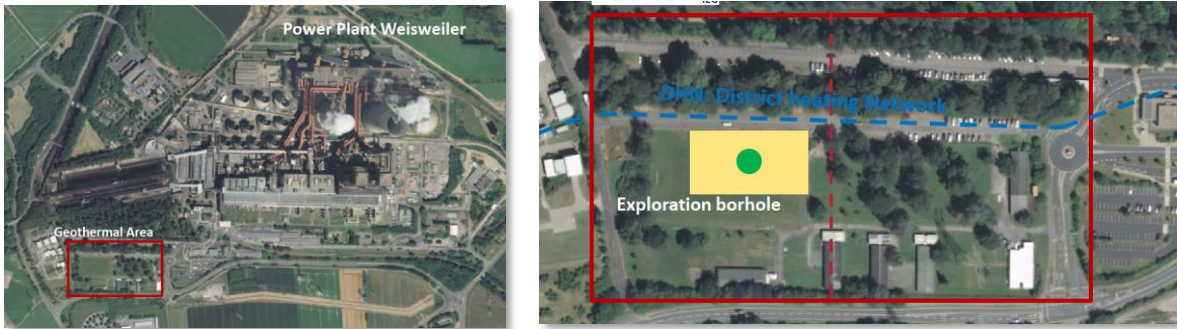
Figure 2: Location of the geothermal area SW of RWE's lignite power plant Weisweiler (left); the western part of the geothermal area will be used for a drilling campaign by Fraunhofer IEG and RWE and form the basis for a field laboratory and full-scale demonstrator of DGE exploitation and grid implementation (right). The main pipeline for district heating (blue) can be easily reached.
