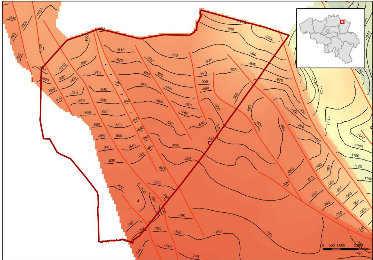
Figure 21: Map of the depth of the top of the Buntsandstein Formation (based on G3D v3.0)
