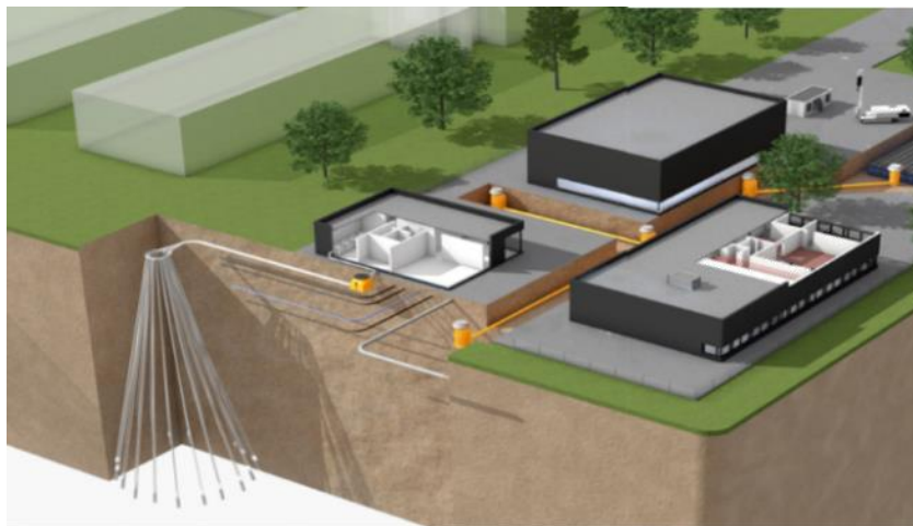
Figure 7. Bochum demonstration site. Left: Set-up of the BTES system GeoStar connected to the campus infrastructure at Fraunhofer IEG.
