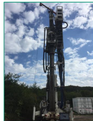
Figure 16. Injection, production, monitoring wells sites (left). Drilling operations with BO.REX ring
