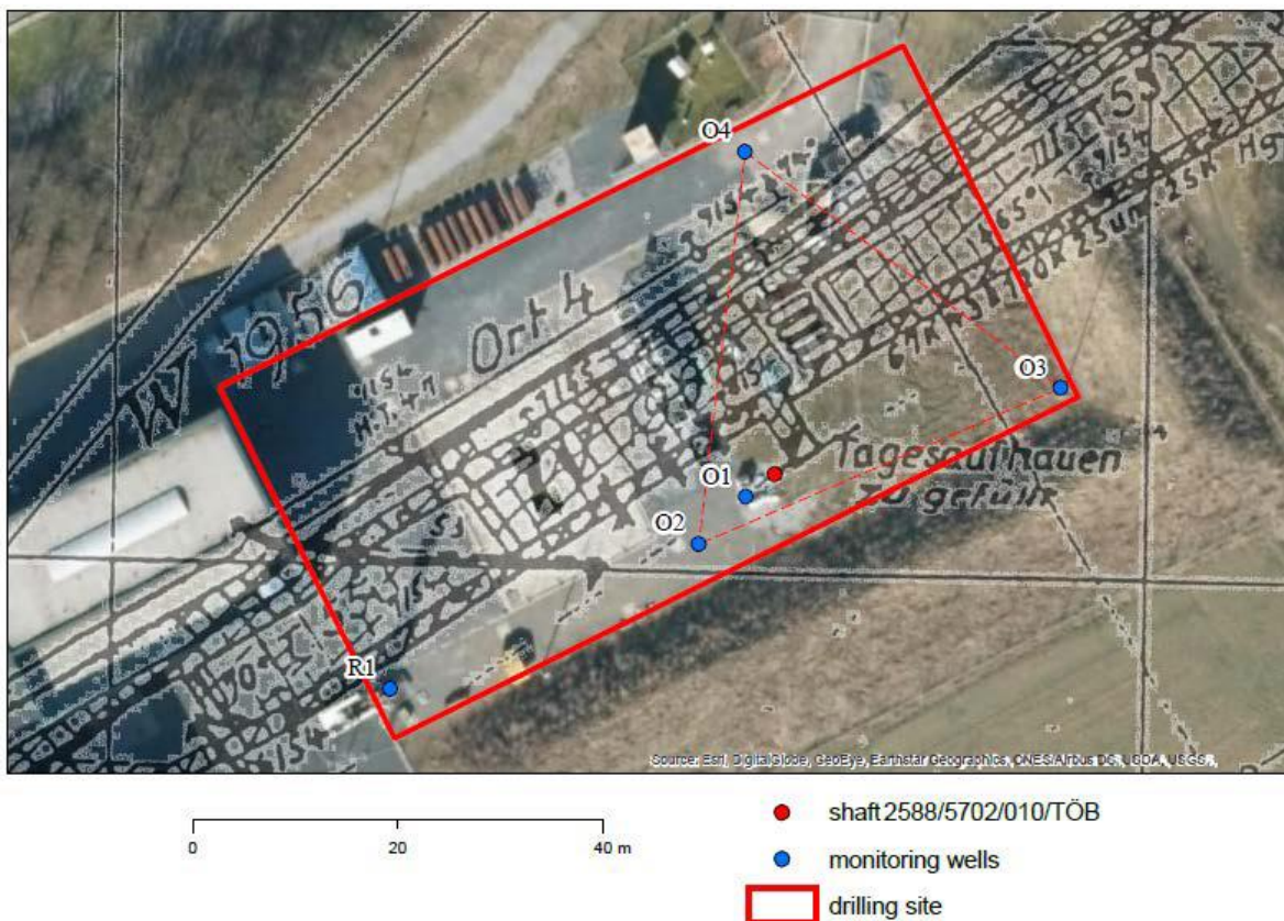
Figure 9. Extent of the abandoned mine displayed on top of the campus pictures.
