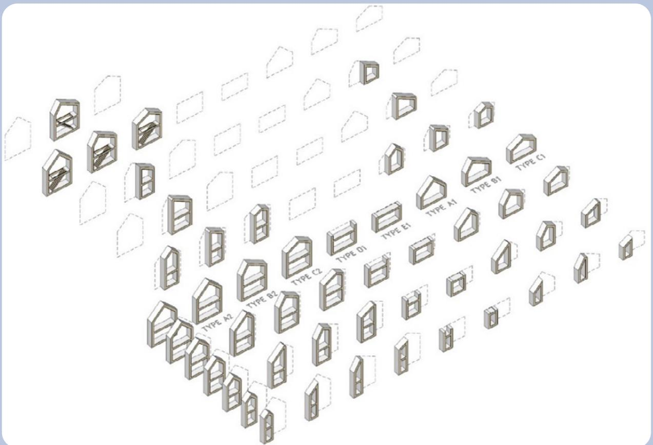
Figure 8: Example of the Toolbox With Standard Modules Available for Self-builders Through WikiHouse
