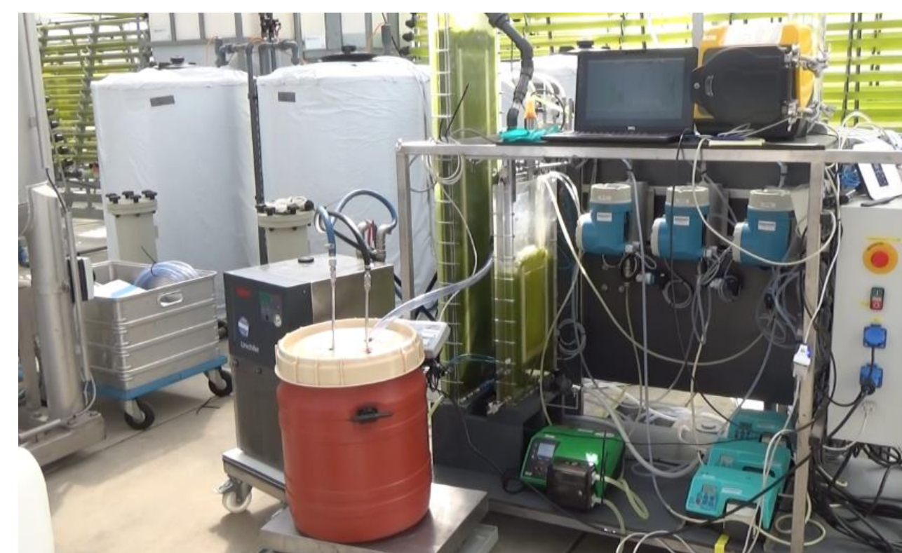
Algae preconcentration by membrane-filtration
