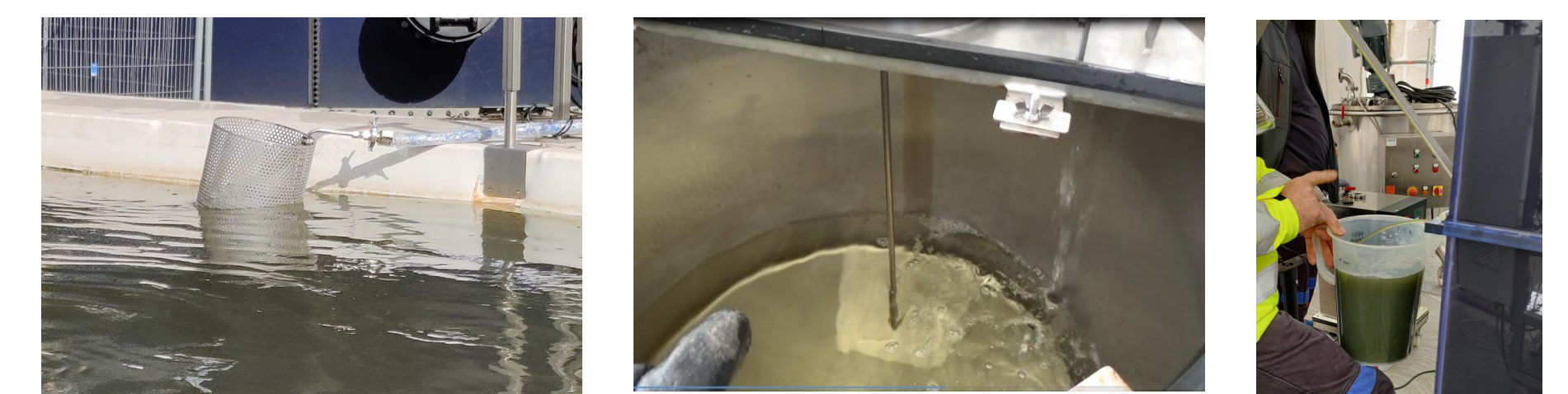
Figure 3: Extraction point of algae suspension from the open pond (left), clear MAF-permeate (middle), algae biomass sampling from MAF (right).
