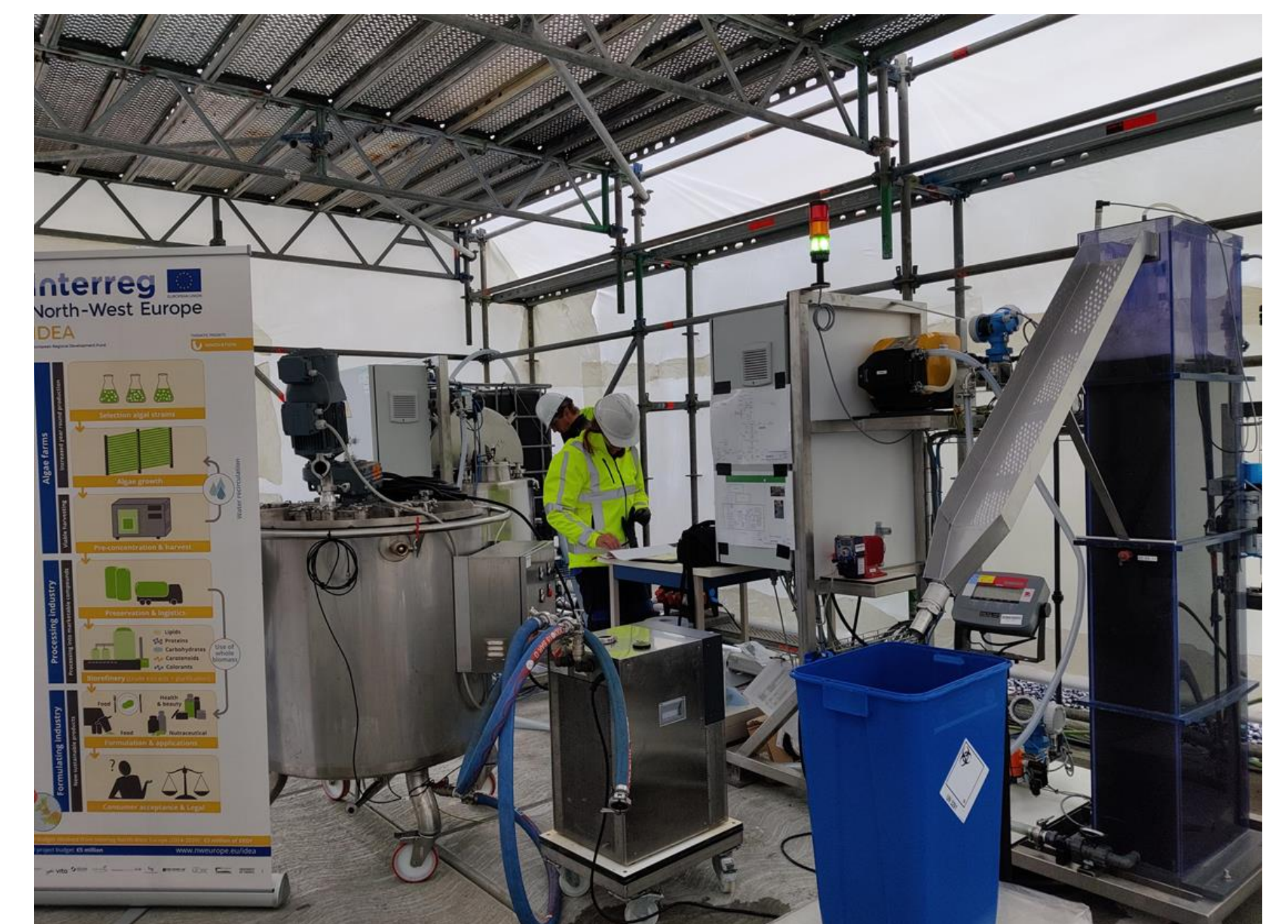
Figure 2: Pilot MAF-harvesting equipment in shelter near algae pond, comprising MAF-device (right) & cooled storage vessel for AMF-concentrated algae (left).
