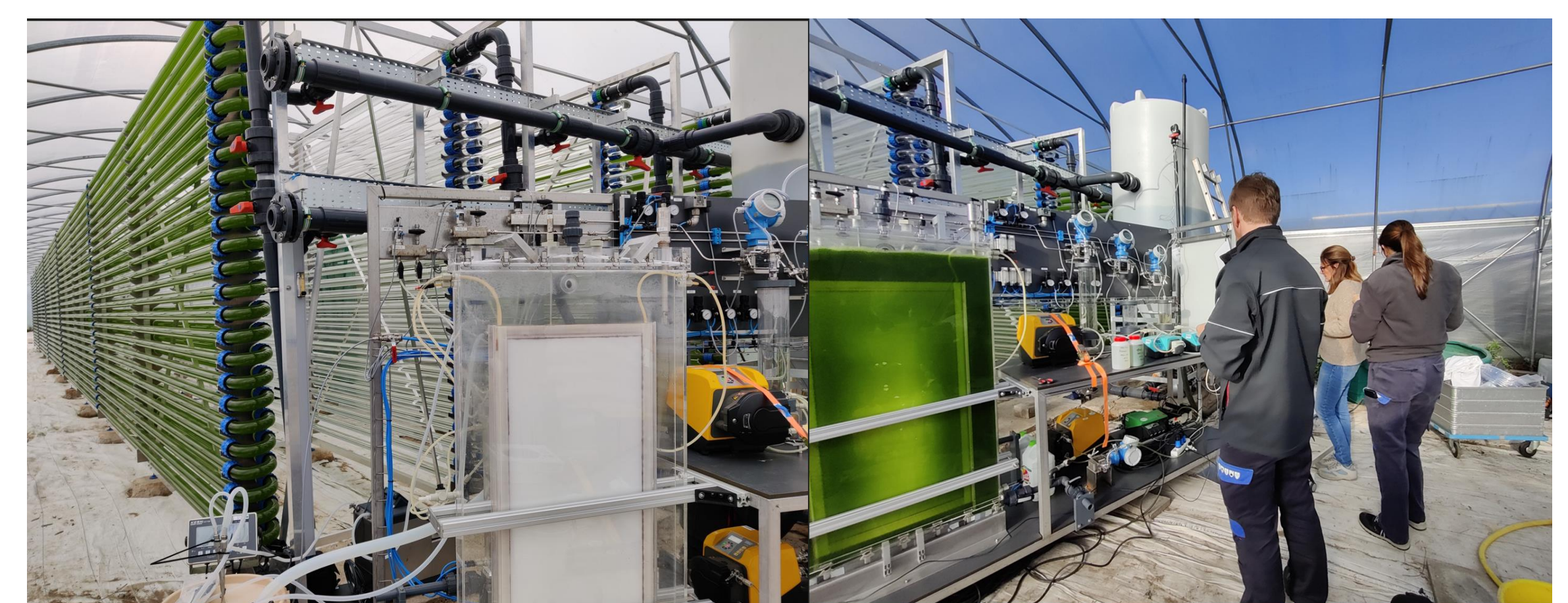
Figure 3: Tubular bioreactor linked to MAF-harvest unit.
