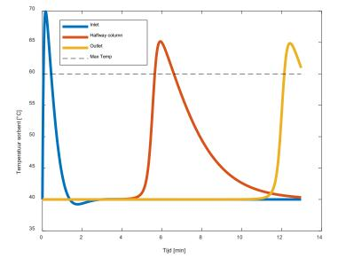
During adsorption a temperature front moves through bed. Re-use of  $\Delta H_{Ads}$  is key
