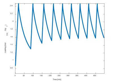
Development of a cyclic steady state. Trade-off between cyclic capacity and maximum T in bed.
