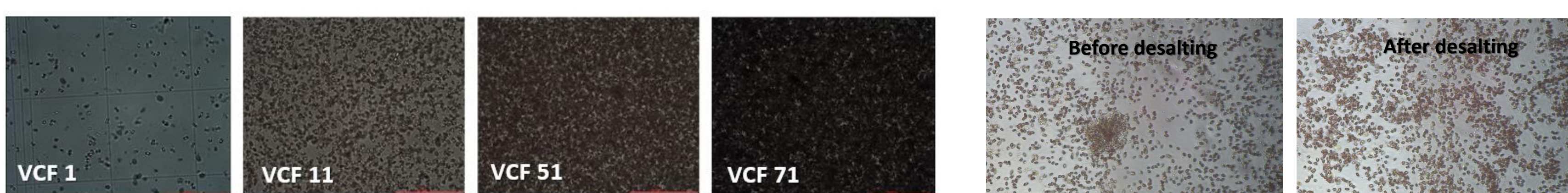
Figure 3: Microscopic analyses of Rhodomonas cells during concentration by MAF till VCF > 71 (LEFT) and before and after desalting (RIGHT).
