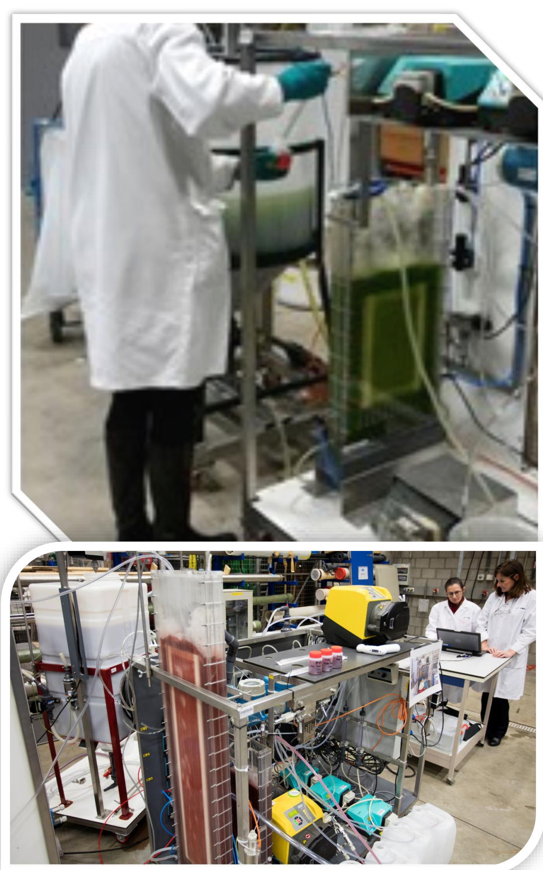
Figure 2: MAF screening units with 0,2 – 1,1 m 2 membrane surface.
