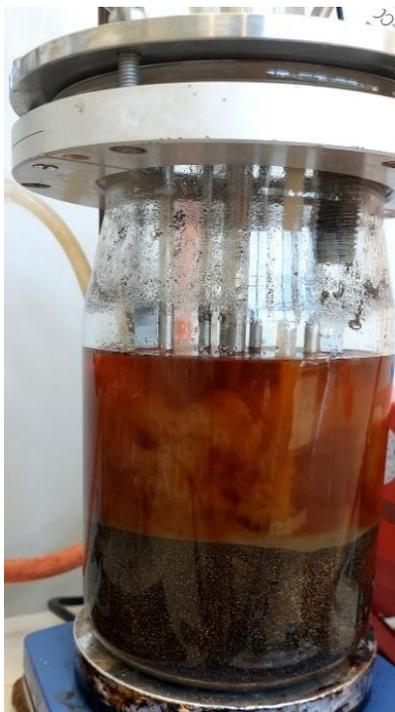
Figure 5-8: Glass reactor in settling phase after a cycle of extraction.
