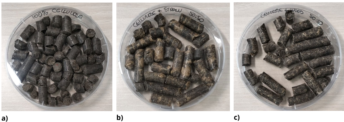
a) Pellets of 100% cellulose, b) 50% cellulose-50% straw c) 50% cellulose-50% wood
