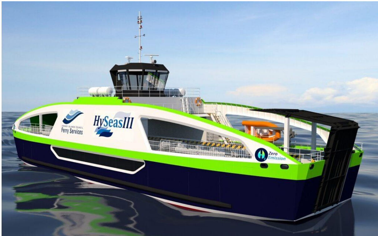
Figure 9 Concept design for European's first hydrogen powered ferry (courtesy of HySeas III)
