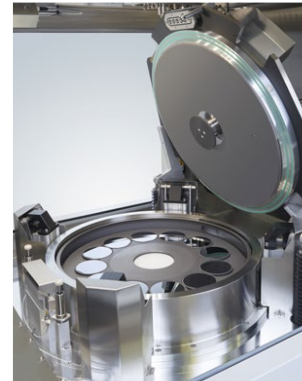
MOCVD (Metal Organic Chemical Vapor Deposition) deposition system for the deposition of semiconductor layer structures on 4 inch wafers.
