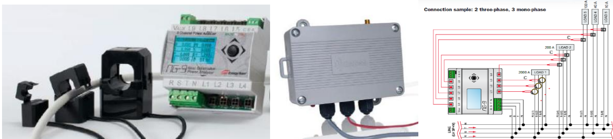
Figure 14: (a) Electrical meter; (b) Associated transmitter; (c) Setup example
