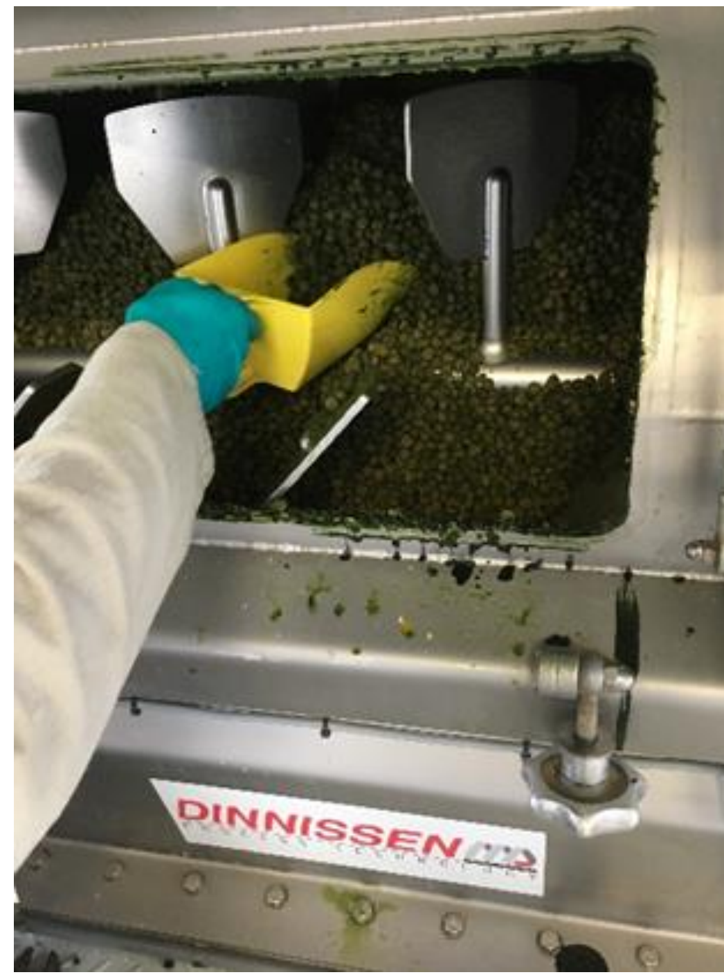
Sampling extruded feed after vacuum coating with wet algae
