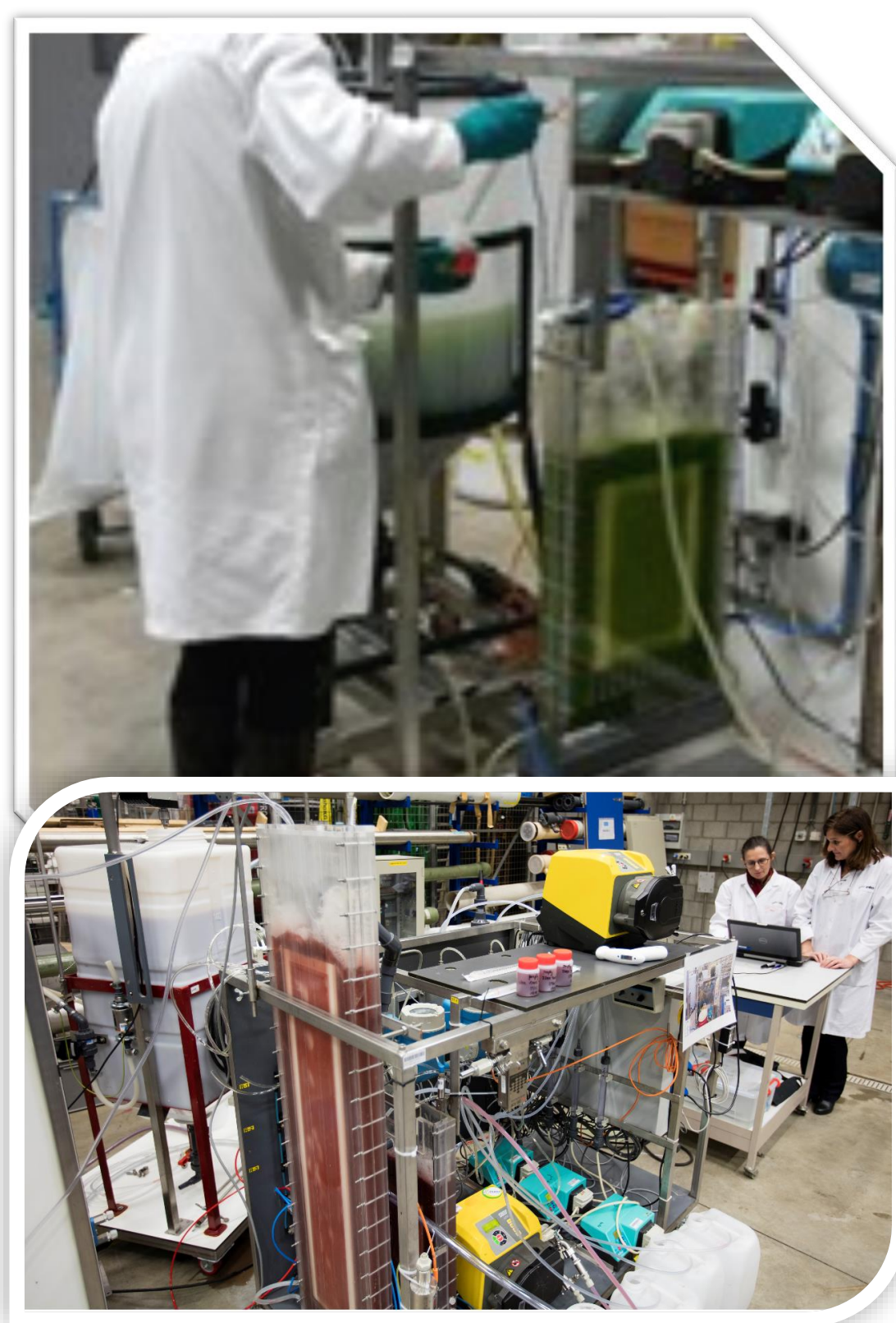
Figure 2: MAF screening units with 0,3 – 1,3 m² membrane surface.
