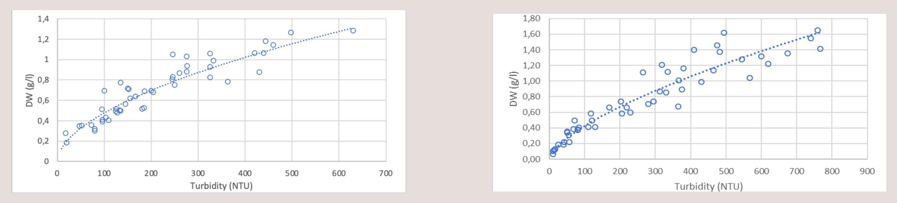
The left figure shows the correlation between the NTU value measured by the online turbidity instrument (X-axis) and the dry weight (Yaxis; g/l) obtained by taking samples throughout the growth period of *C. typhlos* in the photobioreactor. The right pictures shows the graphical representation of the correlation between the NTU and DW for *P. purpureum*.
