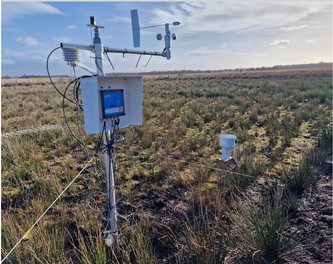
Figure 9. The CGHG monitoring set up, showing the GHG flux measurement equipment and the weather station. The control plot is shown overleaf, and highlights the difference between the carbon farm and adjacent agricultural grassland.
