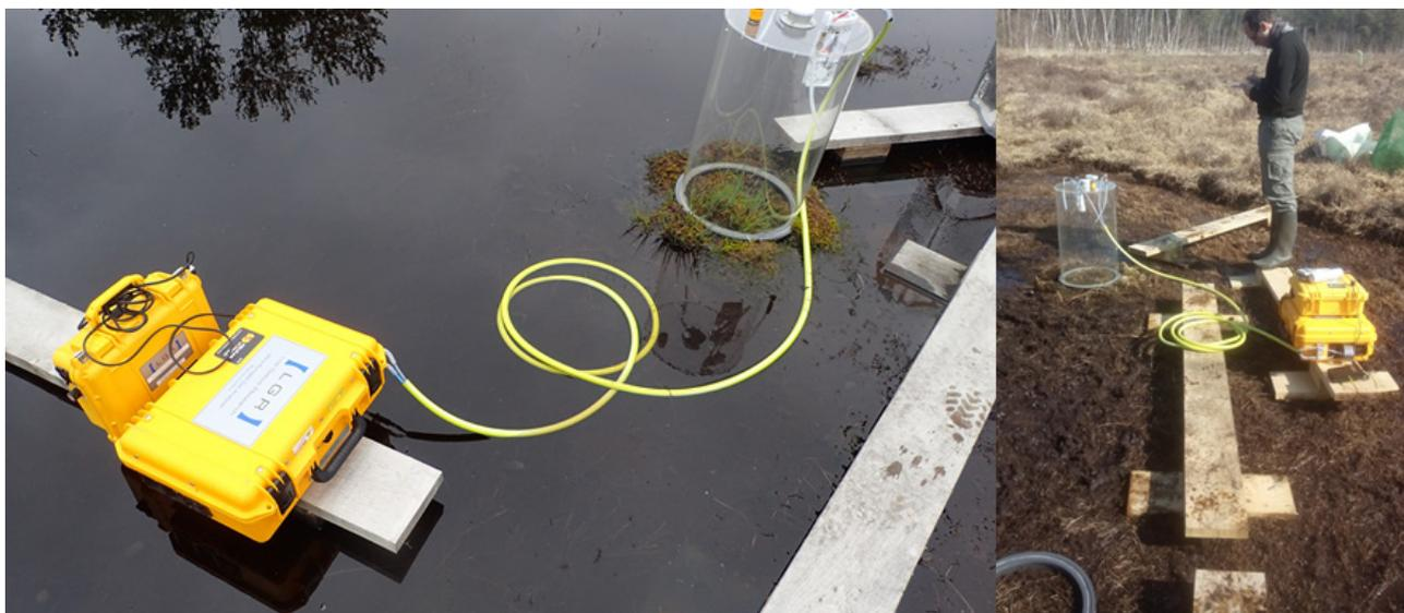
Figure 11. Examples of GHG flux measurements with the operator and the equipment installed on the walk-board.
