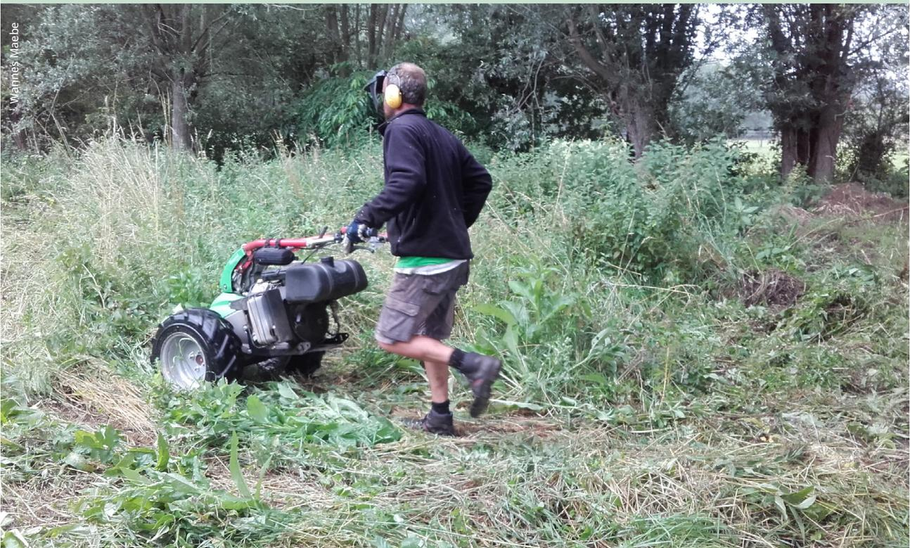
Two-wheel tractor, used on large sensitive parts in the valley.
