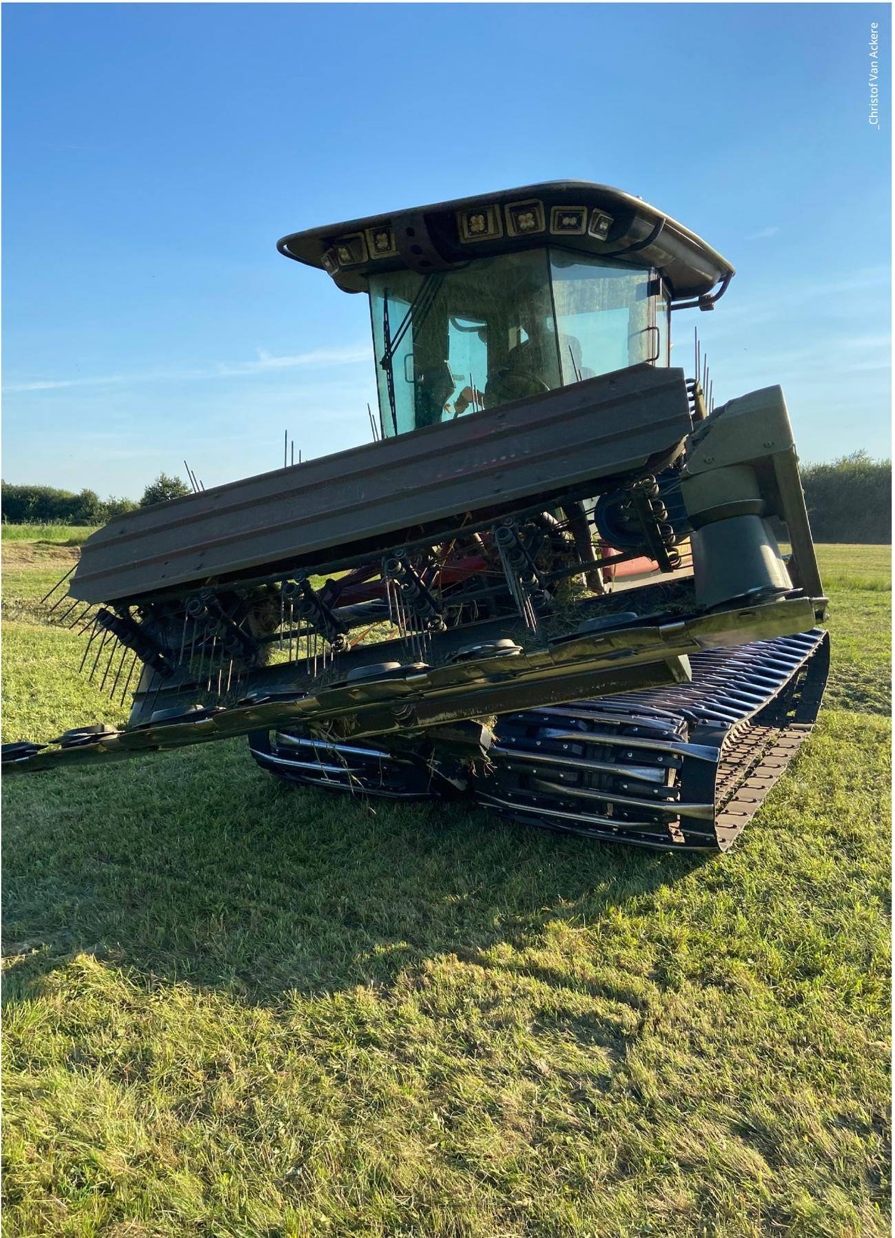
Front view of the track mower equipped with cutter bar and belt rake.
