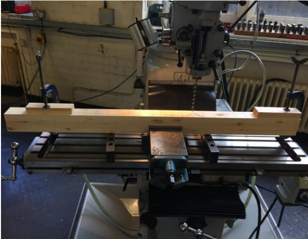
Figure 3. Image showing the AFLT beam setup for drilling
