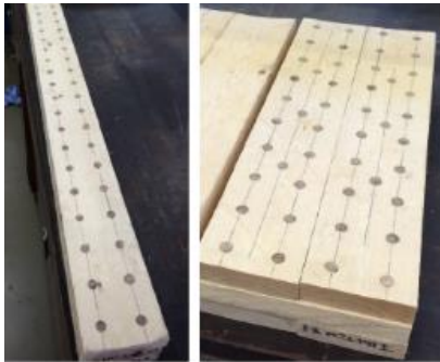
Figure 2: Small beam and CLT panels connected by compressed wood dowels
