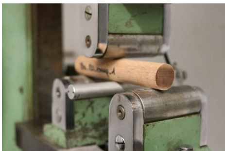
Figure 13. A compressed wood dowel under 3-point bending.
