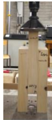
Figure 11. Push-out shear test under monotonic loading.
