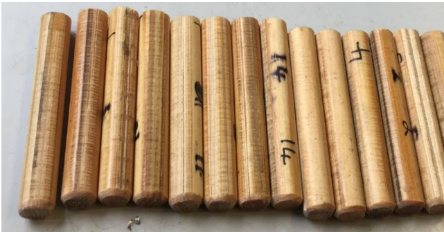
Figure 4. The chamfered compressed wood dowels before insertion into the AFLT beam
