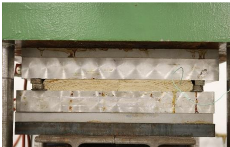
Figure 12. A wood plate is in pressing stage.
