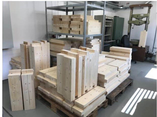
Figure 14. Specimens for push-out tests.
