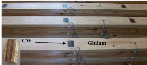
Figure 1: Glulam beams pre-stresses by compressed wood
