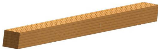
Figure 18. Adhesive free laminated timber column
