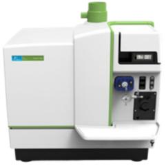
source to create a stream of ions that are measured by their mass/charge ratio in a mass spectrometer. This enables the instrument to measure trace elements in concentrations ranging from ng/l to mg/l. With ICP-OES and ICP-MS we are able to analyse most of the elements in the period table for a wide range of concentrations in water samples.
