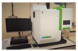
ICP-OES. The Perkin Elmer Avio 500 Inductively Coupled Plasma – Optical Emmission Spectrometer. This instrument is used for analyses of  $\mu g/I$  to percent levels of elements in water. Typical uses are for the analysis of alkali metals, alkaline earth metals, iron, manganese and aluminium or elements that are present in concentrations greater than trace levels. This instrument is installed and awaiting to be comissioned.
