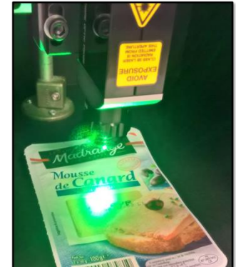
Raman spectroscopy used in the GEPEA laboratory for food analysis.
