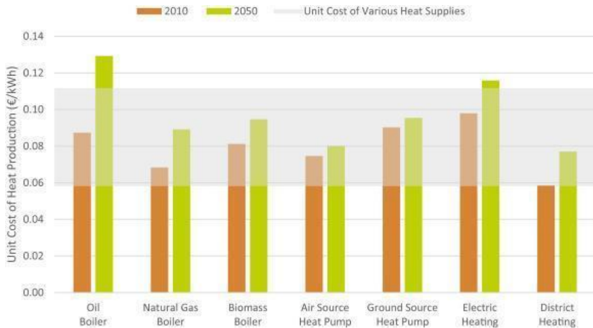
Figure 5: Unit cost of heat production for various heat supply technologies in the years 2010 and 2050 [17]. EU Average and predicted fuel cost are used
