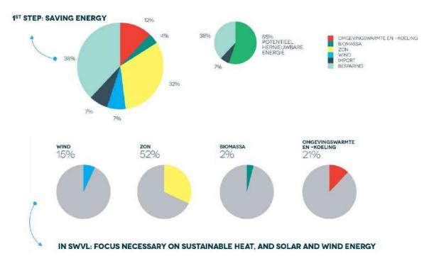
Figure 11: The energy demand will need to decrease by 38% from 2017 until 2050. The potential of renewable energy in 2050 is 91% of the remaining energy demand, namely 4677,83 GWh vs 5141,69 Gwh. Solar energy (yellow) will be the most important renewable energy source compared to wind energy (blue), biomass (green) and ambient heating and cooling (red).
