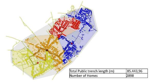
Figure 57: connecting Kuurne to a district heating network requires 15MW heat. The waste incineration plant of IMOG has a capacity of 30MW.
