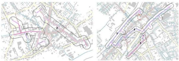
Figure 56: Trajectories of the district heating network in Kuurne (Left) and Harelbeke (Right).
