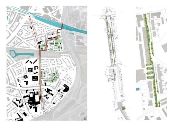
Figure 51: Trajectory of the district heating network in the East of Kortrijk or the 'giant leap'. This trajectory contains public facilities, schools, social housing, ... Cogeneration could serve as a temporary heat source, until the connection is made with the waste incineration plant IMOG. The district heating system could go hand in hand with other climate measures, such as soft mobility (cycling), the greening of streets and water infiltration.
