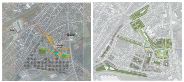
Figure 58: introducing a district heating network in the 'Collegewijk' in Harelbeke, it passes through the neighbourhood and connects the waste incineration plant IMOG with a health care centre and the sport facilities of the municipality. Figure 59: the district heating network stimulates densification of the neighbourhood.
