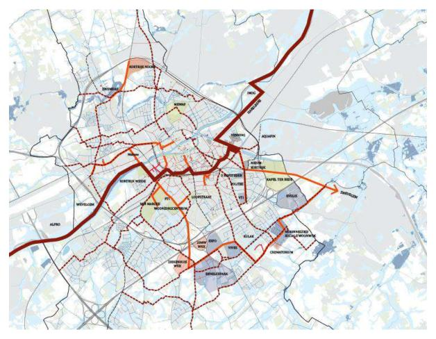
Figure 47: map of the city of Kortrijk showing the expansion of the district heating system: the 'warmteboemerang' (thick dark red line), the current district heating system (red), the expansion of the district heating system (orange). The bicycle network the city of Kortrijk likes to develop (dotted lines) is also an ideal opportunity for grid expansion.
