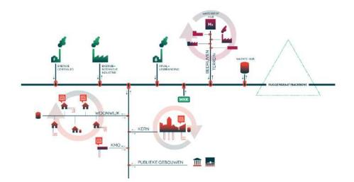
Figure 45: *The 'warmteboemerang' follows the principles of a 4<sup>th</sup> generation district heating network.* Local branches of the district heating network balance heat demand and heat supply. The excess heat of a local branch feeds the 'warmteboemerang', making a balancing of the system possible on a larger scale level.
