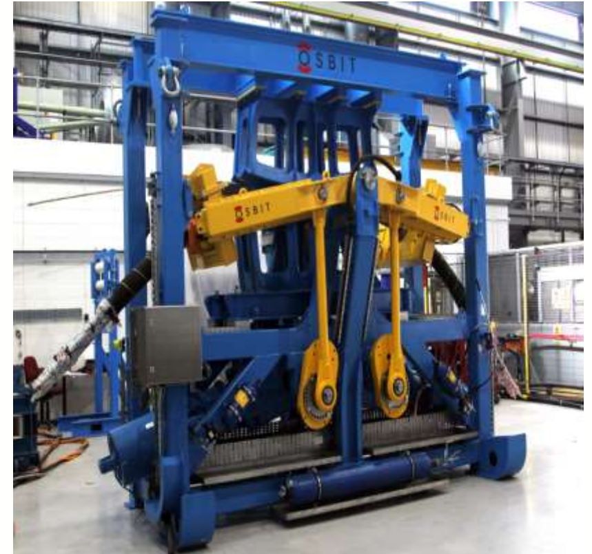
Future work is envisioned to validate models using the new dynamic cable test rig
