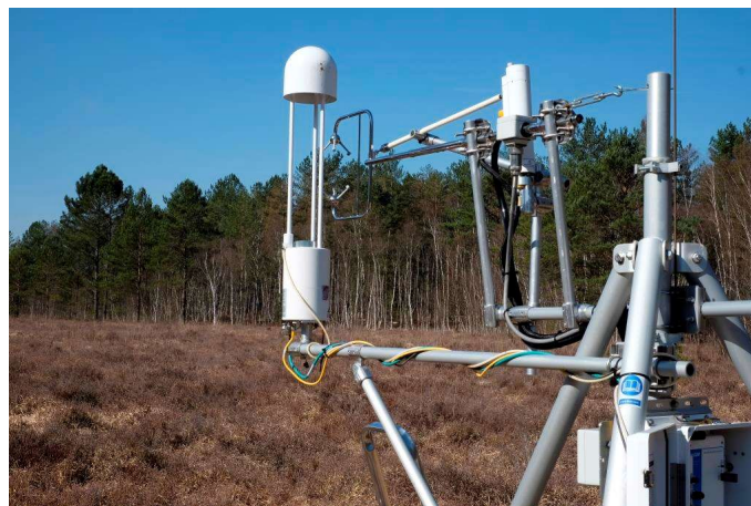
Figure 12 : View of the eddy-covariance station installed on the La Guette site.
