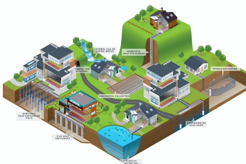
Figure 2 : Different types of near-surface geothermal heat exchanging systems. © Alpine Space Project, GRETA
